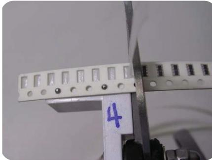
Cut reel using pitch scissors.
