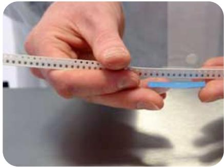
Remove the now joined reels from the splice tool and fold the clear side of the tape over the joint to affix the new and old reels together.
