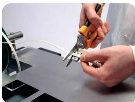
When attaching a new reel, use the hand held splicing scissors to cut straight across the reel ensuring an accurate locating position for both reels.
