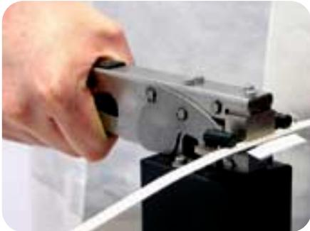
Compress the handles of the splice tool, until it clamps the splice clip.
