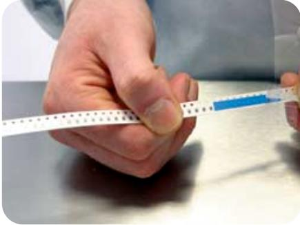
Remove the backing material and observe a perfect and reliable joint.
