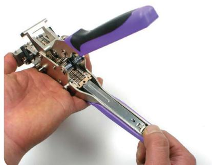
Push the button when the insert clip is inside the guide rail, insert the clip by lifting avoiding the hooked protrusions.
