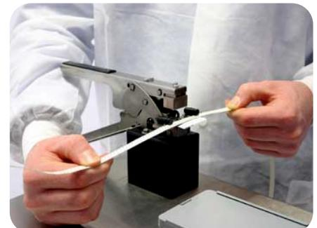
Place the beginning of the new reel on to the placement pin on the right side of the splice clip.
