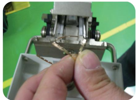
Push the remaining frame forward and remove the frame.
