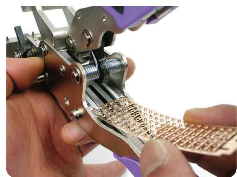
Insert clips into the inside rail. Be careful not to damage / bend the frame.
