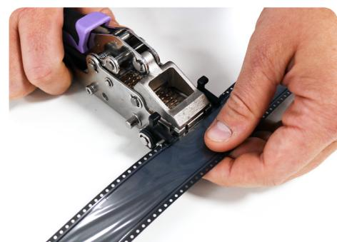
Place the carrier reel tape into the gauge pins, fix the lever and compress.
