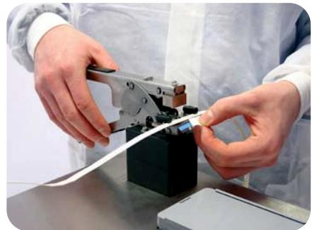
Remove the backing material from the splice tape and discard.
