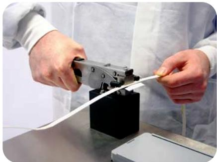
Place the end of the old reel on to the placement pin on the left hand side of the splice clip.
