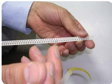
Peel off the reel cover tape. to the first component.
