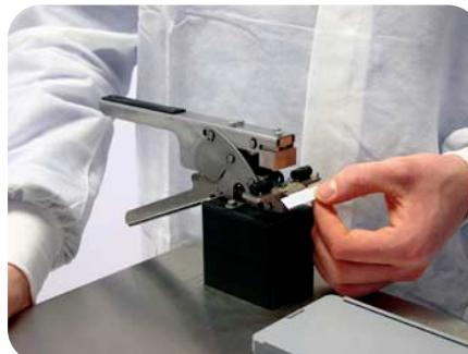
Place the splice clip onto the locating pins of the splice tool, so that the clear film points away from the splice tool, and the backing material faces upwards.
