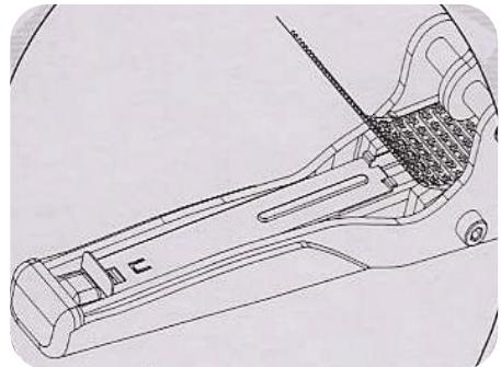
Please be careful when inserting the frame so that it does not bend and ensure the frame is in the correct position.
