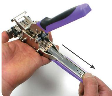
Pull the slider towards the direction of the arrow.
