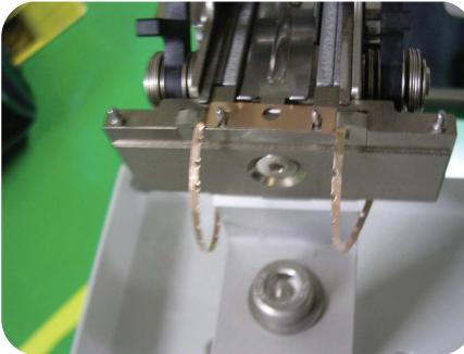
After splicing the final clip check the remaining frame. All clips should be used as per the picture. If there are any clips left then extra care should be taken when removing them from the frame.
